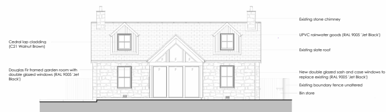
6 Proposed South Elevation 1 : 100
