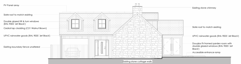
7 Proposed West Elevation 1 : 100
