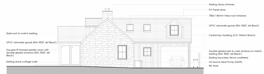
5 Proposed East Elevation 1 : 100
